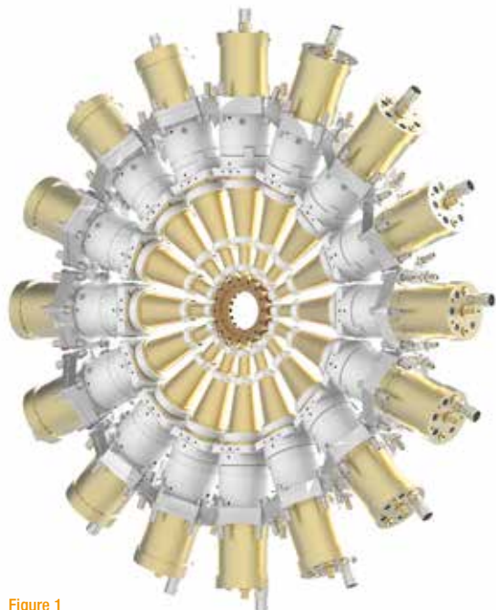
Figure 1 The employed angle-resolving spectrometer built at beamline P04 at DESY. Copyright Frank Scholz.
