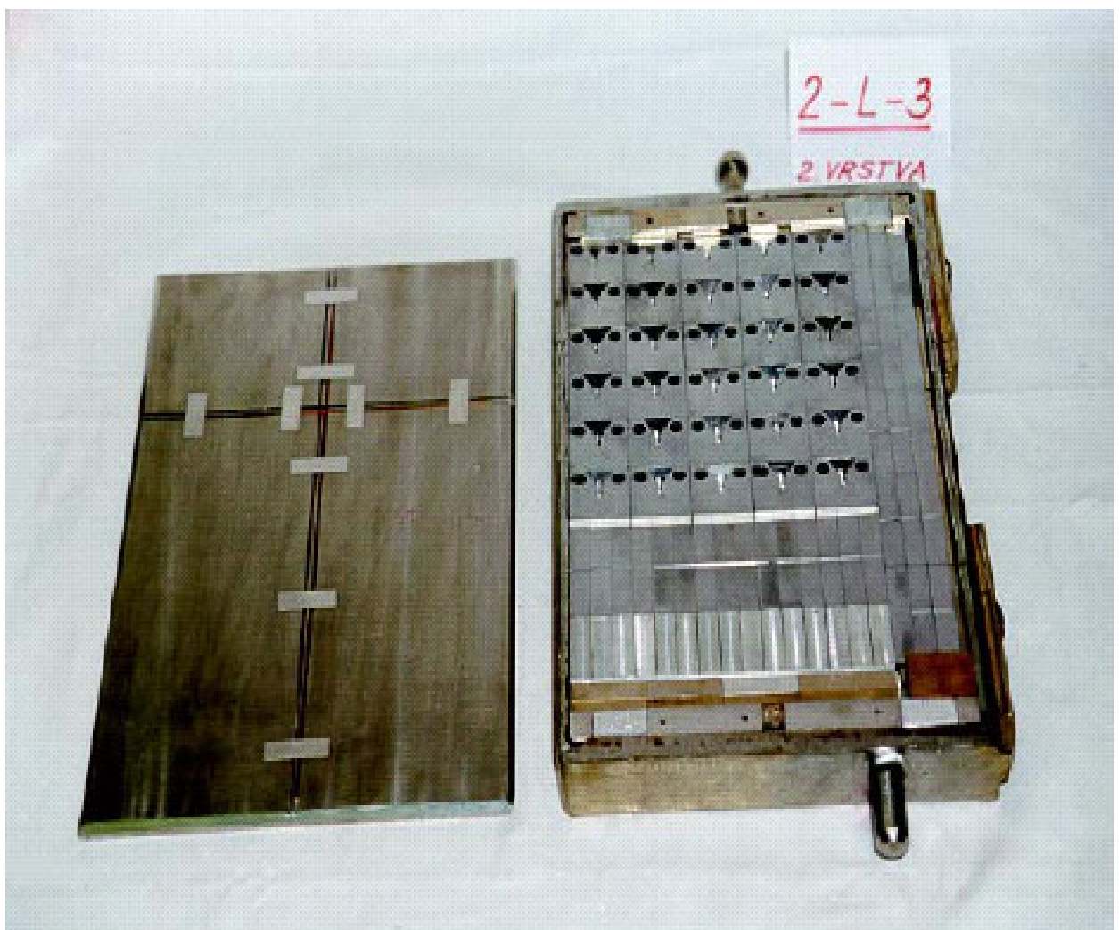
Fig. 50. Picture of an opened container with specimens (right) and neutron wire monitors (left) for WWER-1000 RPV Modified Surveillance Programme
