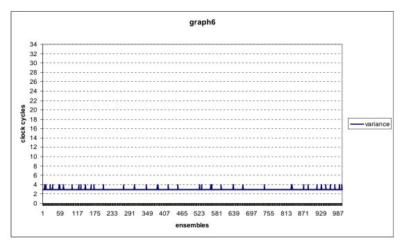
In <u>Figure 5</u>, we can see how the minimum value is perfectly constant between ensembles. In <u>Figure 6</u>, we have the variance being either equal to 3 or 4 clock cycles.
