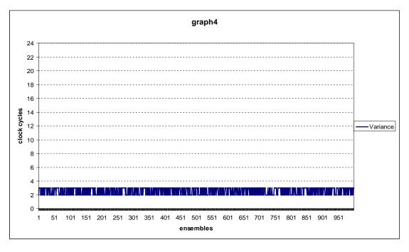
In <u>Figure 3</u> we can see that the minimum value is perfectly constant between ensembles; in <u>Figure 4</u> the variance is either equal to 2 or 3 clock cycles.
