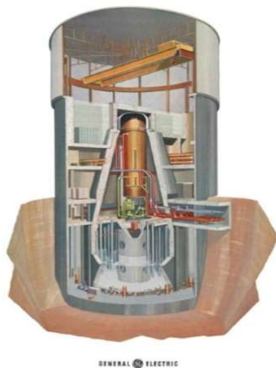
FIG. 1. Scheme of MARK II containment [1].
