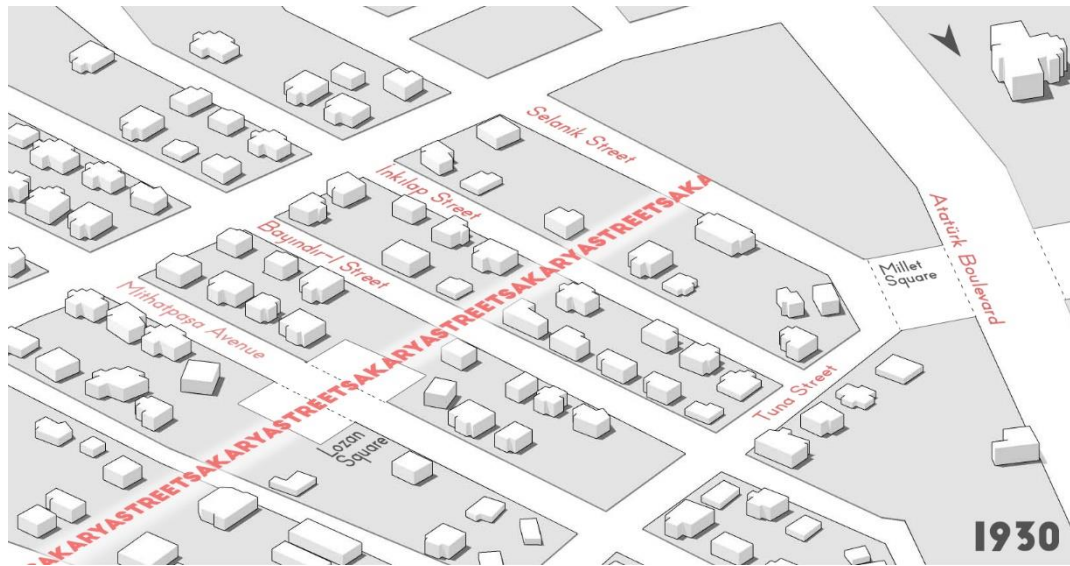
Figure 3.63 Axonometric view of the urban form of Sakarya Street and its surroundings in 1930, built in the light of the Lörcher and Jansen Plans. Kızılay Building and Kızılay Square are on the upper right, and Sakarya Street is not yet in contact with Atatürk Boulevard. Modeled and visualized by the author.
