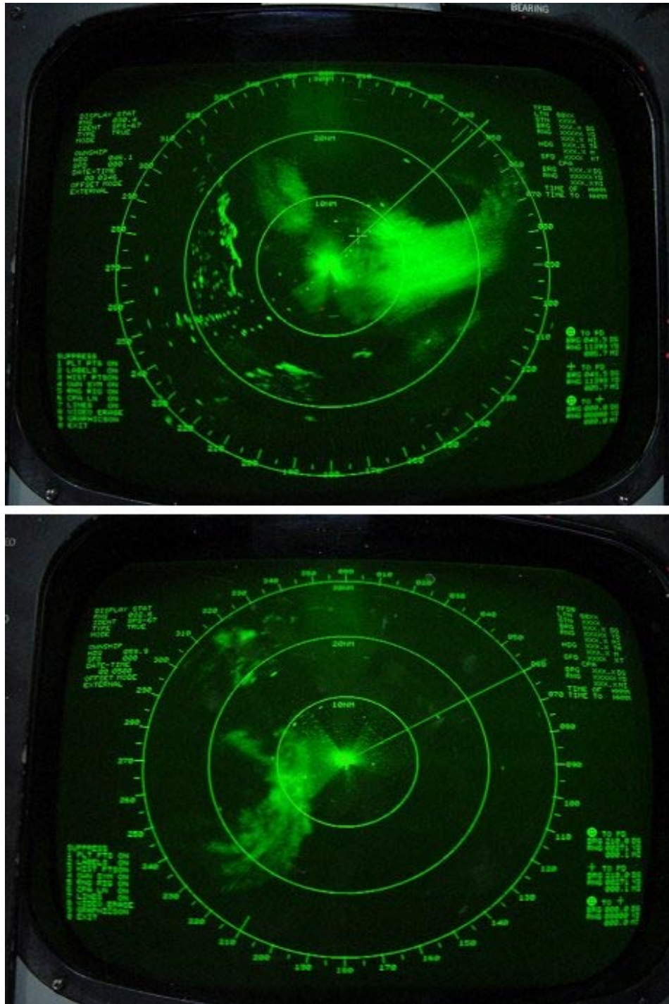
Fig1-32W-4. The top image is the radar depiction of the eye of TY 32W (Vamei) to the northeast of the USS Carl Vinson as the ship moved towards the storm center. The bottom image depicts the eye feature to the southwest of the USS Carl Vinson as the ship moved away from the tropical cyclone. The ships meteorologist indicated that the USS Carl Vinson passed south of the cyclone eyewall and had that feature (eyewall) continuously depicted on radar until the ship passed the center.
