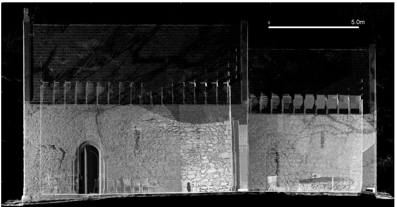
Figure 45: Laser scan images of Cruggleton Church; (above) isometric view from SW, (below), S elevation.
