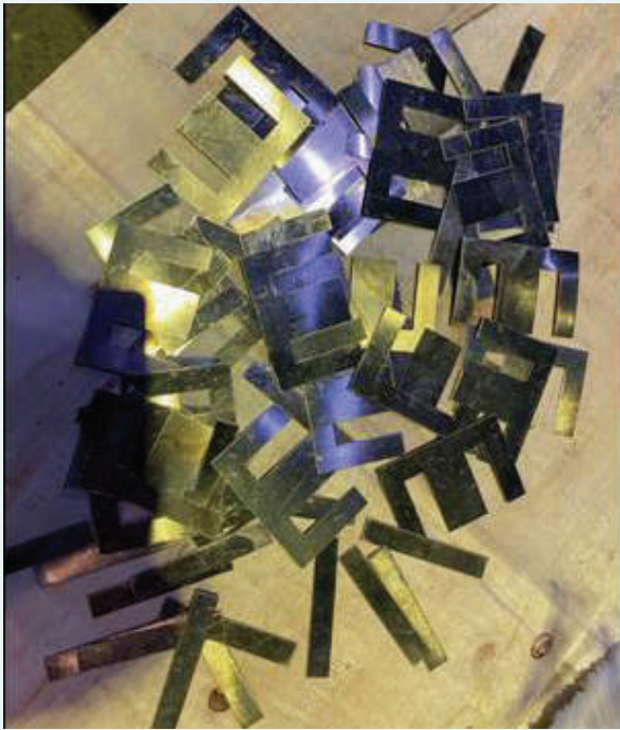
'E' & 'I' shaped laminates made of gold
