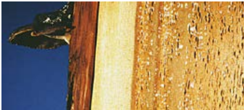
Figure 252. Longitudinal section depicting pockets of mycelia which form in late decay stage.
