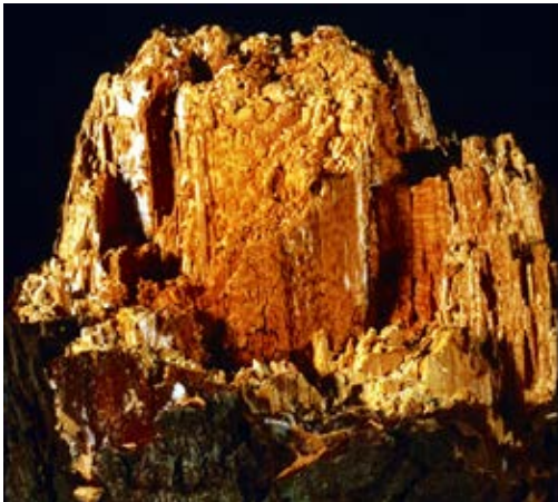
Figure 233. Advanced decay of Douglas-fir by F. pinicola . Note brown cubical rot and white mycelium in the cracks of decayed wood.
