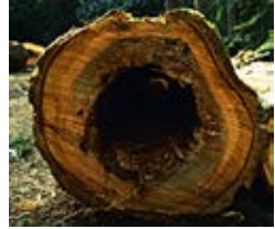
Figure 255. Disintegration of the heartwood in the butt of a Douglas-fir caused by Phaeolus schweinitzii .
