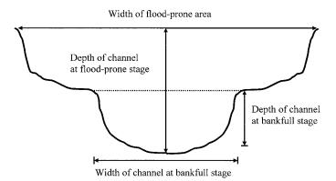
Figure 2. Entrenchment Ratio and Width to Depth Ratio. Entrenchment ratio is defined as the width of the flood prone area divided by with width of the channel at bankfull stage while the width to depth ratio is defined as the width of the channel at bankfull stage divided by the average depth of the channel at bankfull stage.
