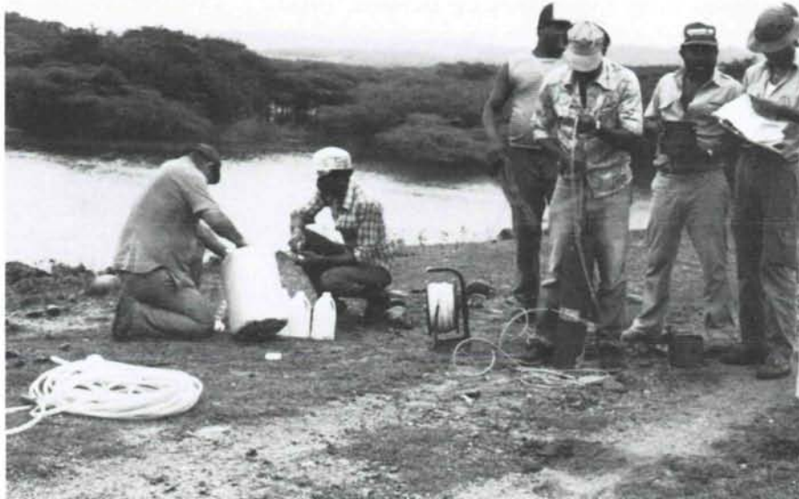
Investigation of dam seepage at the Maguaca reservoir, Dominican Republic.
