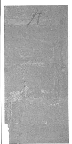
**Figure 15 -**Full depth beam flexural crack.
