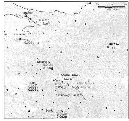
**Figure 3** - Peak ground accelerations recorded from the Mw = 6.3 event (indicated in gray) and from the Mw = 6.0 event (indicated in black).
