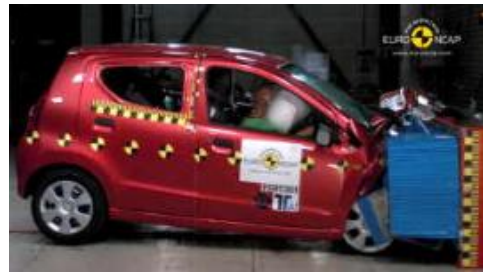
Offset crash test at 64km/hr
