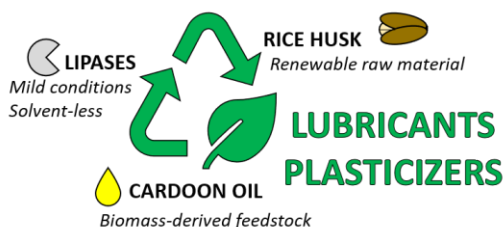
Figure: “Green process” to obtain bioplasticizers and biolubricants starting from cardoon oil.
