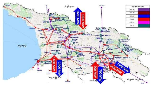
Fig. 1.15 Cross-border transfer capacities between power systems of Georgia and its neighboring countries as for 2031
