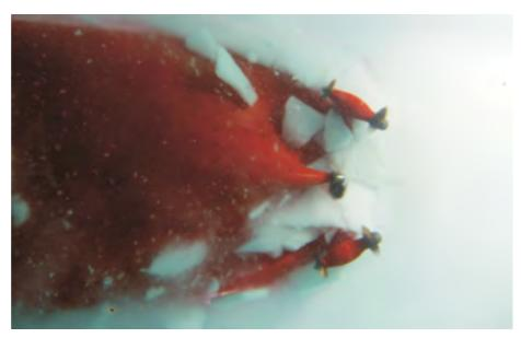
icebreaker, for large size LNG carriers, and most recently in offshore support vessels for verifying the expected higher ice management efficiency. In all ice operating cases the energy saving efficiency has been proven. In these cases the icebreaking capability appears to be improved, but different types of thruster installation will be required compared to traditional thrusters.
