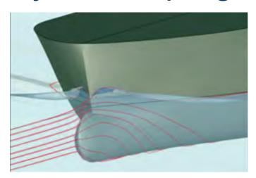
With the new Computational Fluid Dynamics program more alternatives can be evaluated in detail before open water model tests.
