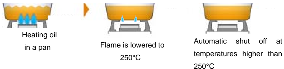
Fig. 3 Schematic diagram of flame control
