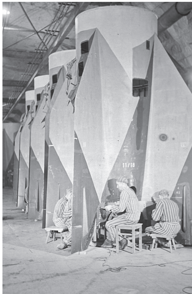
Mittelbau prisoners work on the tail assembly of the V2 rocket, possibly in Hall 35, 1944.
