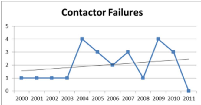
Figure 43 Total contactor faults across entire fleet
