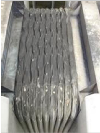
Figure 87 Image of inter-car gangway bellows
