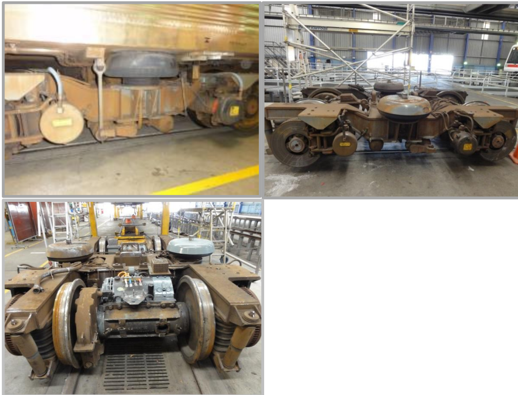
Figure 59: Image of bogie and secondary suspension
