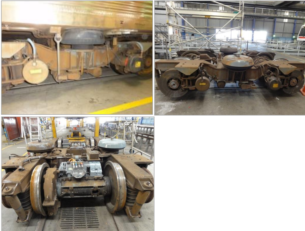
Figure 59 Image of bogie and secondary suspension
