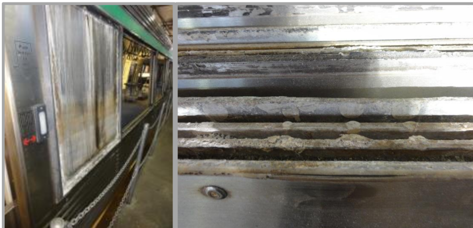
Figure 71: Image of door push button release and de-lamination of leaf aluminium skins
