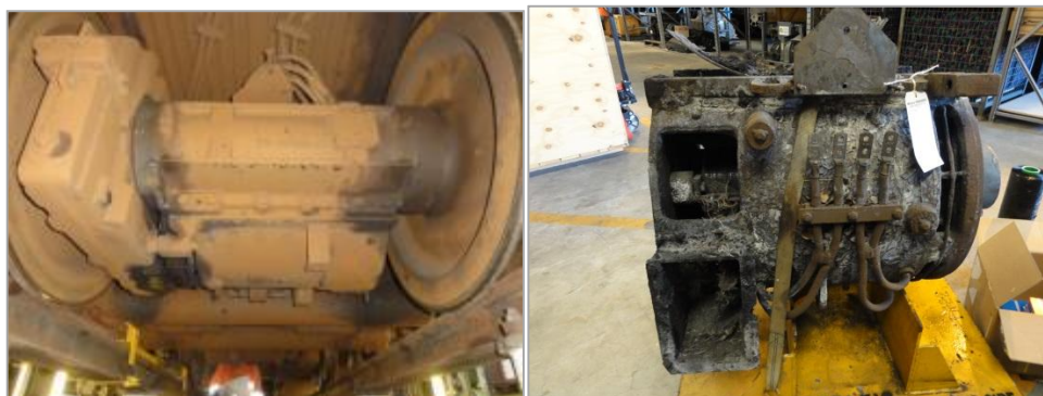
Figure 47 Image of traction motor and a burnt traction motor that occurred during operation
