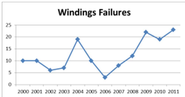
Figure 46 Total windings faults across entire fleet
