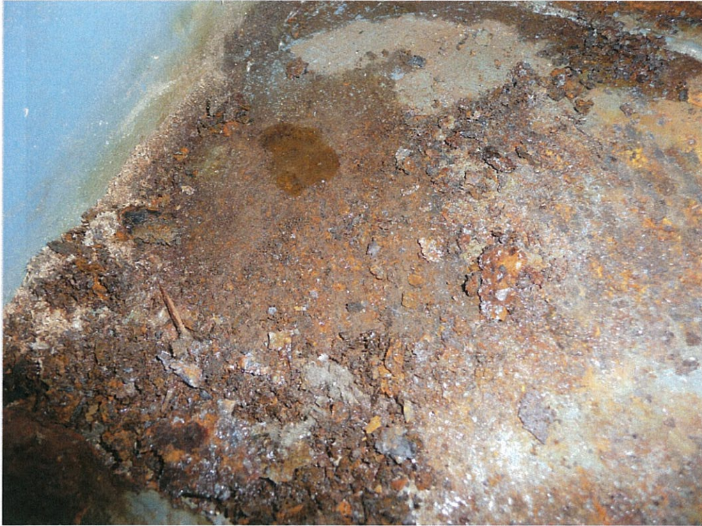
Figure 4: Area of corrosion on the headstock floor on EMU 23
