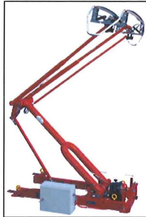
Figure 16: Air Cushion Pantograph
