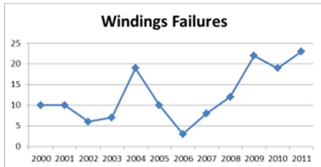
Figure 46: Total windings faults across entire fleet
