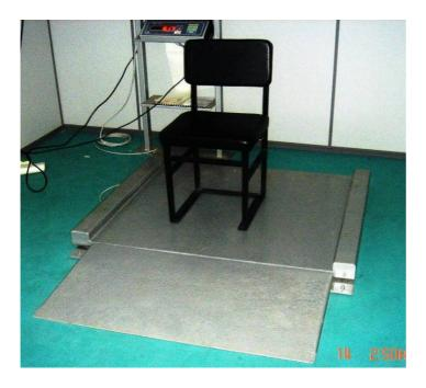
Example of electronic digital scales. The scales can be used with or without a chair.
