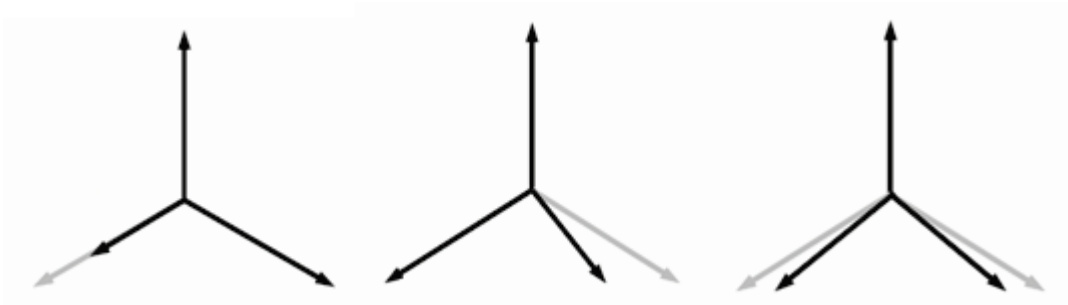
Figure 6-1 Testing vectors 3A, 3B and 3C according to IEC 61000-4-34.
