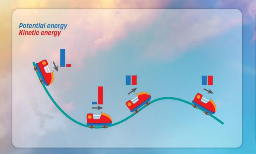
The roller coaster car gains Gravitational Potential Energy (GPE) as it travels up the lift hill.
