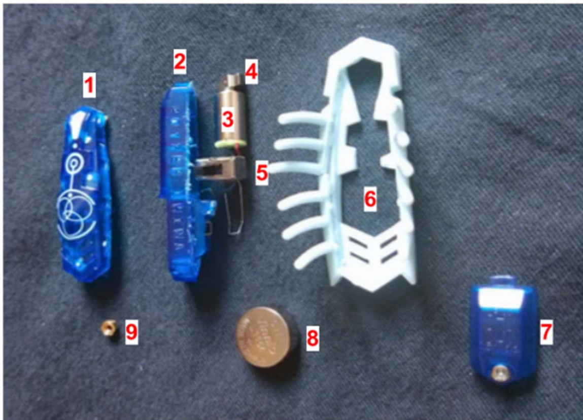
Figure 52. Hexbug Nano fully disassembled
