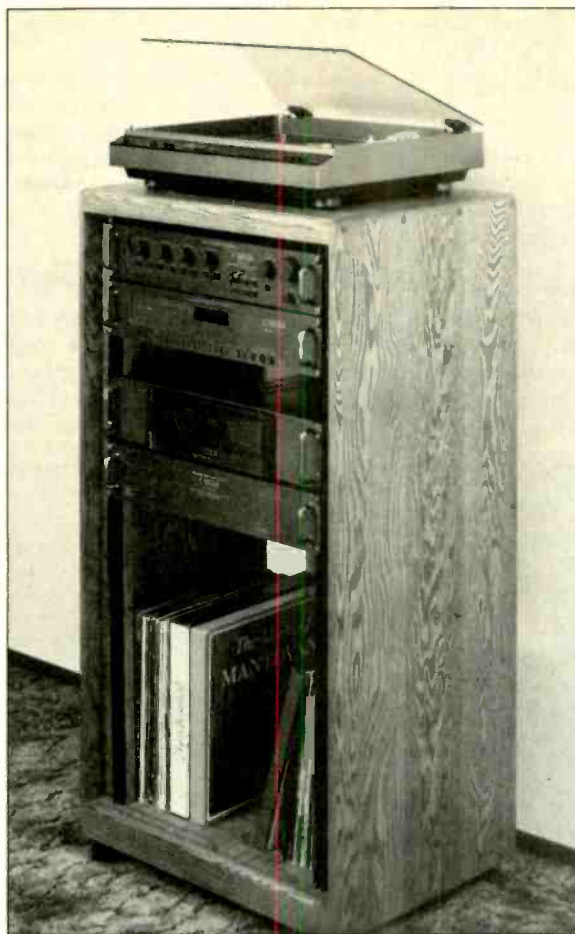
The 19-inch front-mounting rack system in this cabinet from Sunrise Audio Systems obviates the need for shelves, which can take up usable space and block ventilation. Note the gaps left above and below the power amplifiers so air can flow around them for cooling.
