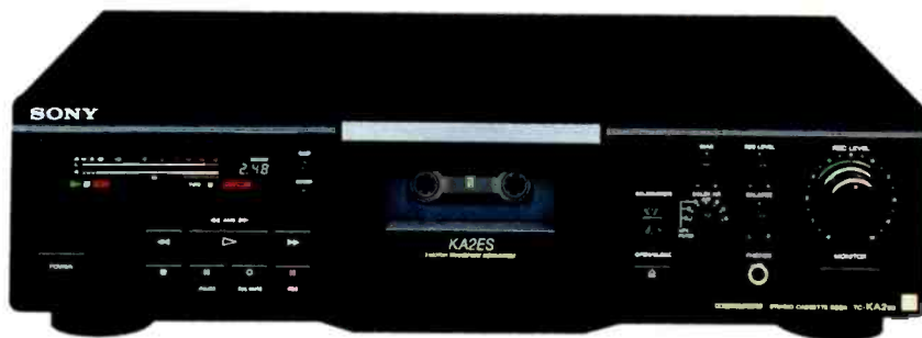
Sony's TC-KA2ES ($550) is a three-head deck with a three-motor, dual-capstan transport, Dolby S, B, and C and HX Pro, and sixteen-segment peak-level metering.
