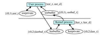
Fig. 3. Information interaction between user process and operating system
