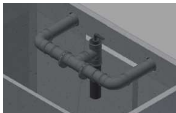
Fig-8: allocation device and the primary filter in a septic tank
