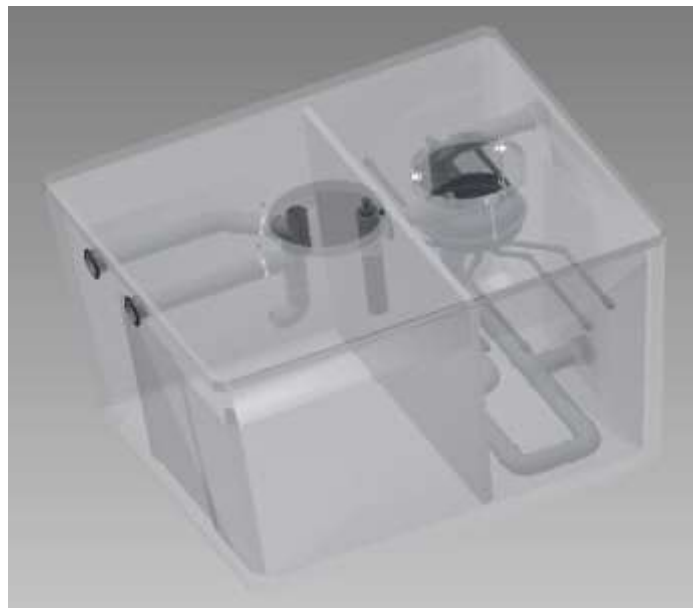
Fig-2 : Operating Principle of the X-Perco® C-90 5PE single tank (view from the primary settling tank)
