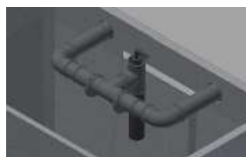
Fig 34 : Allocation device in the septic tank
