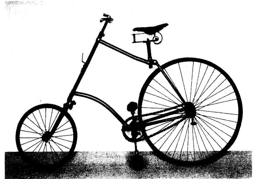
Figure 2.22 From 1884 to 1886 several new designs were developed, in various aspects widely different from the basic scheme of the Ordinary bicycle. The Humber “Dwarf Safety Roadster,” also designed in 1884, had a trapezoidal frame. In their model of 1886, Humber introduced a front fork with the forward bending of the Singer 1878 bicycle. Photograph courtesy of the Trustees of the Science Museum, London.
