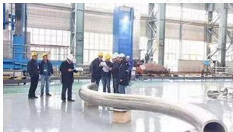
主管道及波动管 Main-pipeline and Surge line
