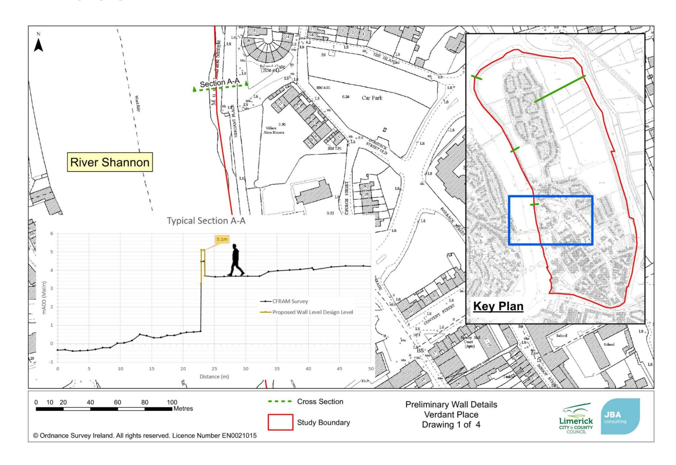
The plot above shows the Verdant Place quay wall at its current height (in black) and gives and indication of the height the flood relief wall would need to be (in orange). The proposed wall could be about 0.6m above the existing wall.
