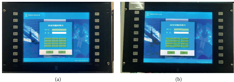
FIGURE 12: Physical picture: (a) SVDU physical equipment; (b) SVDU simulator.
