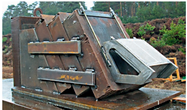
Protection of modern generations of main battle tanks are simulated by proving ground targets.
