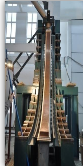
Test of Cavity Injection and Cooling System
