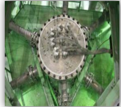
Core Inlet Flow Pressure Drop Test
