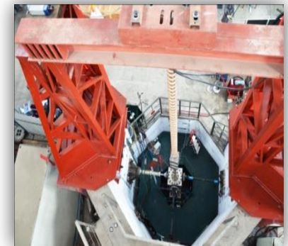
Seismic Test of Control Rod Driven Line (CRDL)
