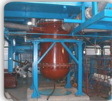
Mixing Tests of Reactor Vessel Down-comer
