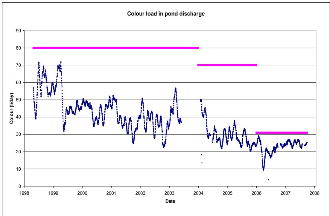
Figure 8 Colour load (tonnes/day) discharged from the Tasman treatment ponds into the Tarawera River with consent limits shown.
