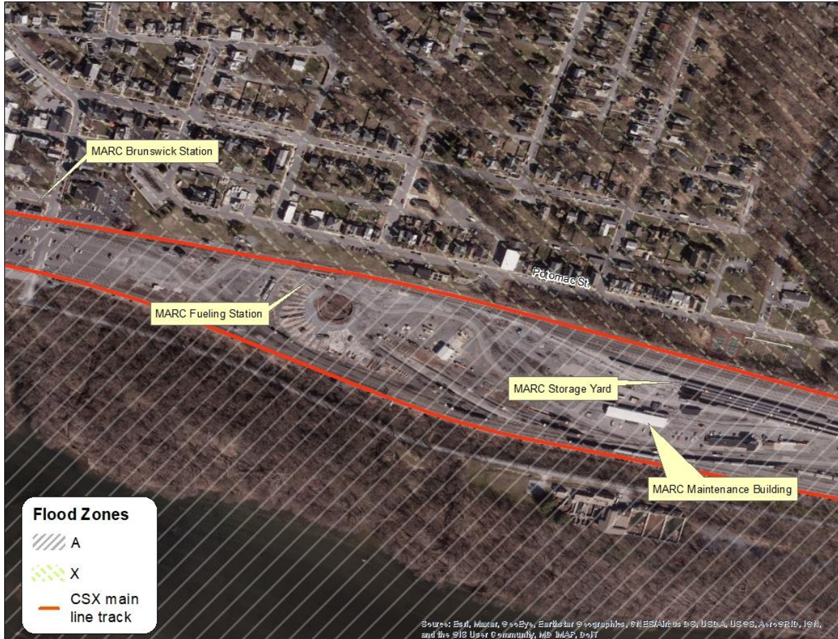
Figure 8 - MARC Brunswick Yard within Zone AE Floodplain
