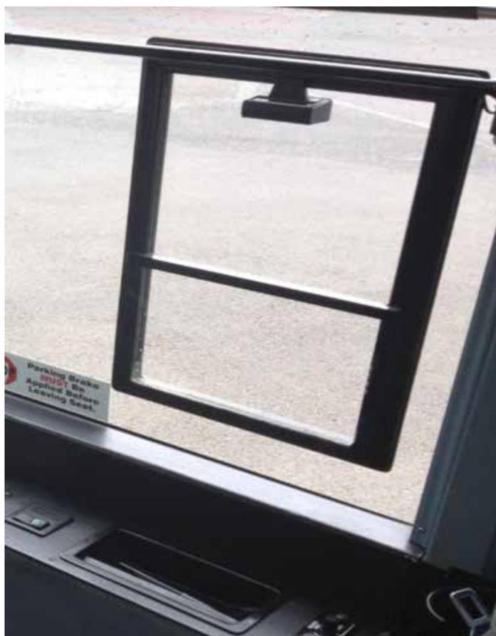
View of drivers' side window which is elevated to prevent access to the door open buttons from outside the bus
