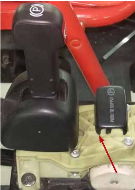
View of broms brake valve and park brake on chassis
