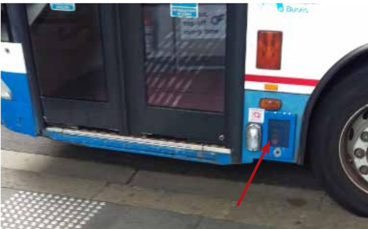
View of glass panel which can be opened in normal situations with a T-key to access the door open close buttons or the glass broken in emergency situations.
