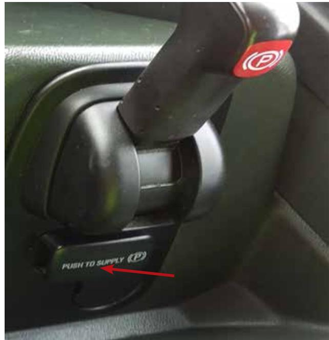
View of broms brake valve and park brake in bus
