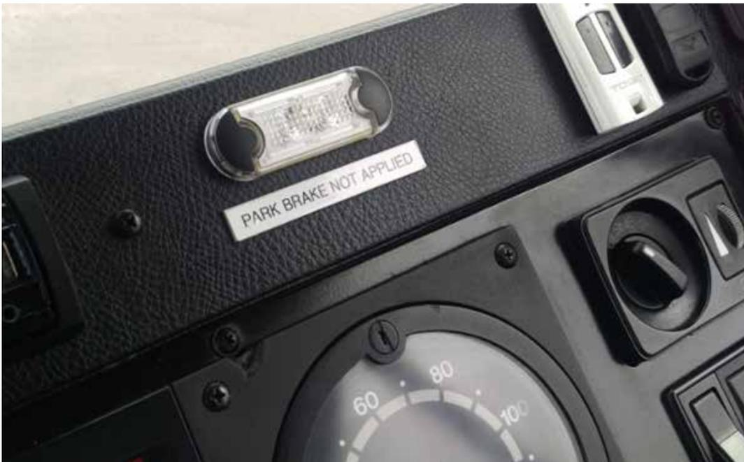
View of retrofitted visual warning alarm that activates if the park brake has not been applied.
