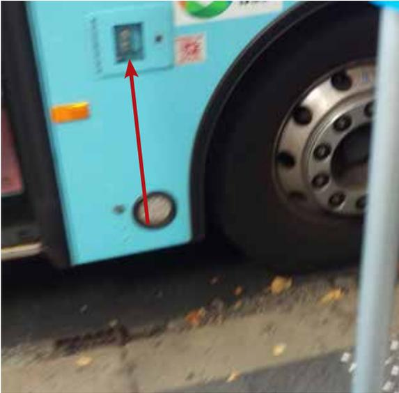
View of glass panel which can be opened in normal situations with a T-key to access the door open close buttons or the glass broken in emergency situations.
