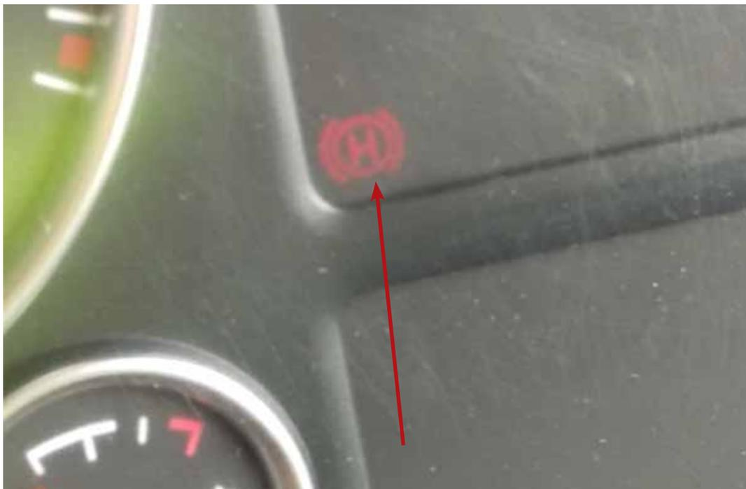
View of the centre console indicator showing that the park brake has not been applied.
