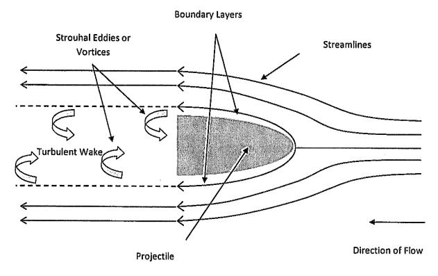
Figure 2. Subsonic Flow Past a Projectile.
