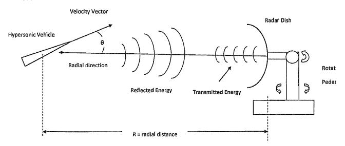
Figure 10. Schematic of a RADAR System.
