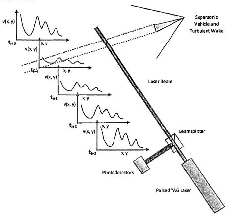
Figure 17. Schematic of a Pulsed LIDAR System.
