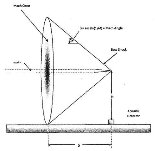
Figure 18. Mach Cone Generated by a Supersonic Object.
