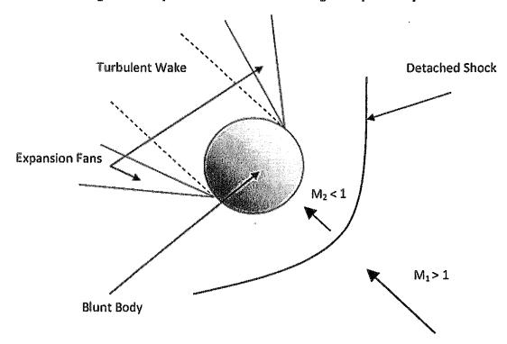
Figure 5. Supersonic Flow Past a Blunt Body (Spheroid).
