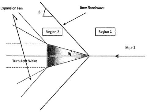
Figure 4. Supersonic Flow Past a Wedge-Shaped Body.
