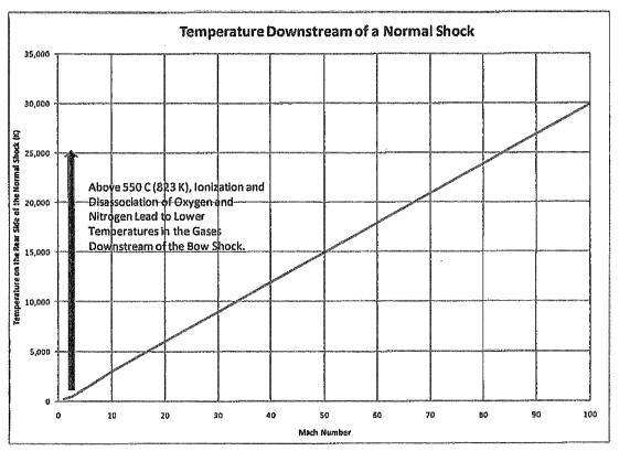
Figure 16. Peak Shock Layer Temperature for Hypersonic Objects.
