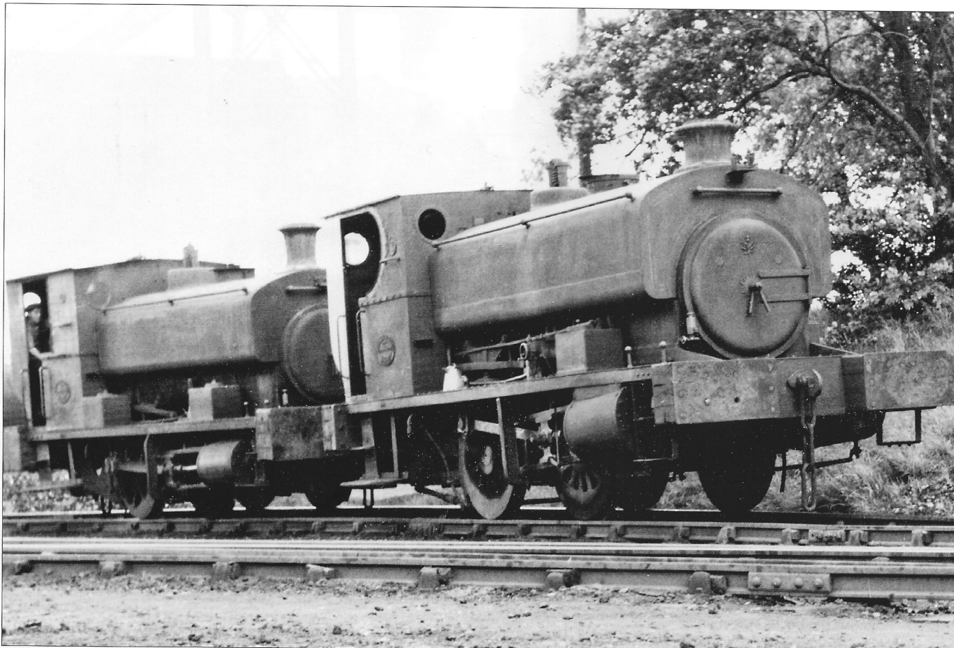
On 11 th June 1960 Barclays Nos. 7 and 10 are at work with the leading loco (probably No.7) lacking a front dumb buffer. Perhaps detail by then ceased to matter! If correct, at the rear is No.10, the escapee, which is currently lodged with the Fife Heritage Rai at Methil. (Photo Kenneth G. Williamson, cty. Hamish Stevenson)
