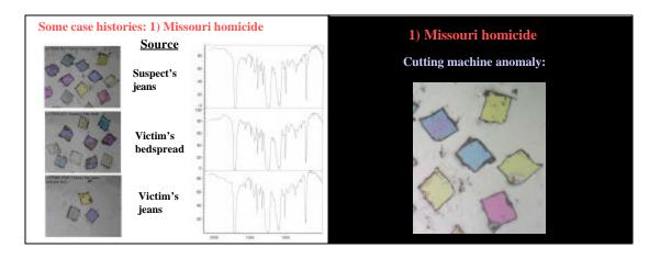
Notice one corner tends to be rounded and an adjacent corner tends to have a protrusion.
