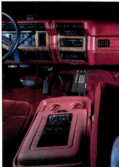
The control section; note the equalizer and individual-speaker switching in the box between the seats.
