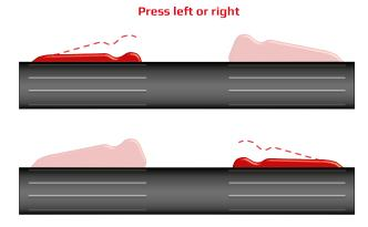
This also means that the propeller will spin as long as the gear is not 0 and at least one button is pressed. This allows for changing the hand that controls the scooter on the way.
