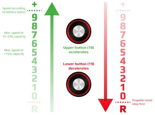
Pressing the top piezo button (drawing 2, pos. 18) causes the gear to move higher and pressing the bottom button (drawing 2, pos. 19) will lower it. Each pressing changes the gears by one step.
