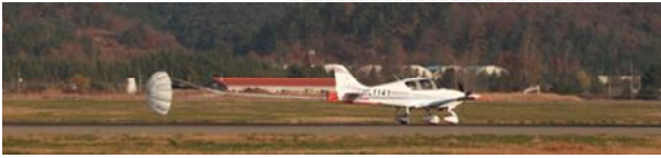
Fig. 2. Taxi Test for SRS Verification
