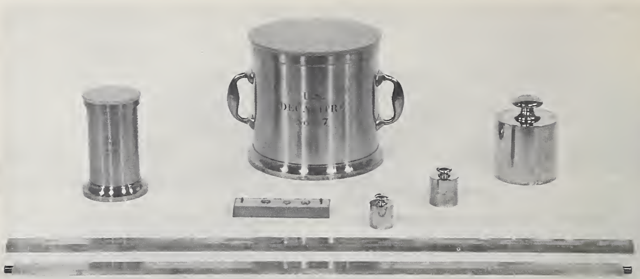
Metric standards of length, mass, and capacity, furnished to the States under the joint resolution of Congress of July 27, 1866.
