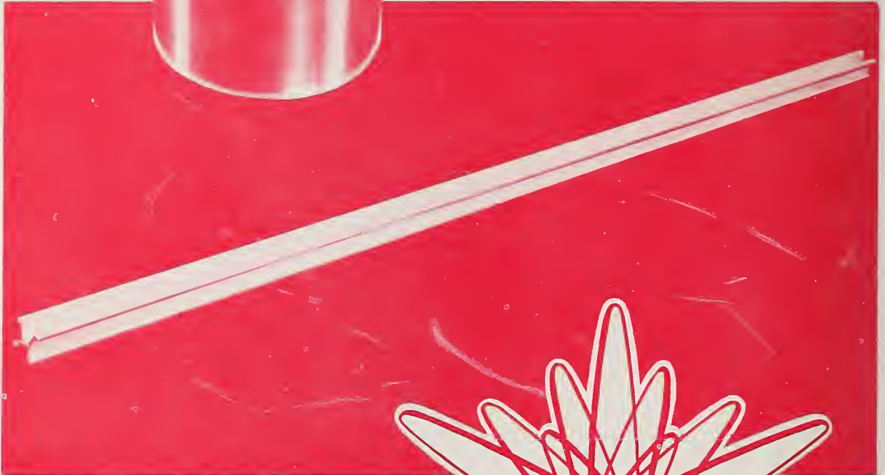
U.S. Prototype Meter Bar 27, the standard of length of the United States from 1893 to 1960. On October 14, 1960, the meter was redefined in terms of a wavelength of the krypton 86 atom.
