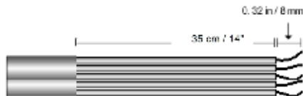
Figure 32: Insulation stripping – AC
