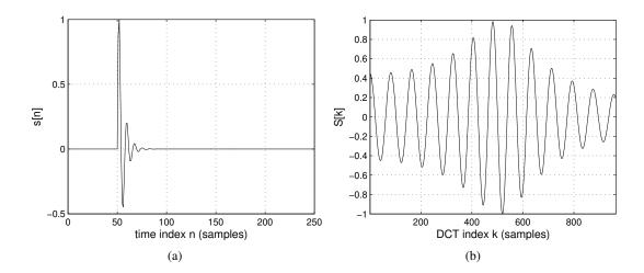
**Figure 2.13:** *Example of DCT mapping: (a) an impulsive transient (an exponentially decaying sinusoid) and (b) its DCT as a slowly varying sinusoid.*
