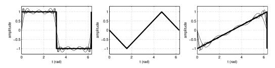
**Figure 2.17:** Bandlimited synthesis of the square, triangular, and sawtooth waves, using 3, 8, and 13 sinusoidal components.
