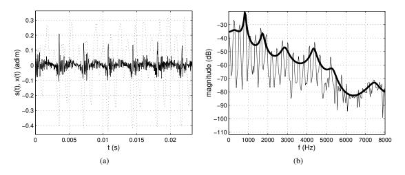
**Figure 2.24:** Example of LP analysis/synthesis, with prediction order p = 50; (a) target signal s[n] (dotted line) and unit variance residual x[n] (solid line); (b) magnitude spectra |S(f)| (thin line) and  $|gH_{LP}(f)|$  (thick line).
