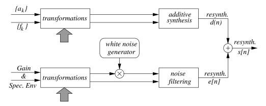
Figure 2.12: Block diagram of the sines-plus-noise synthesis process.
