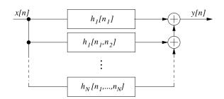
**Figure 2.33:** *Realization of a non-linear system with memory using the Volterra series (truncated at the order N).*
