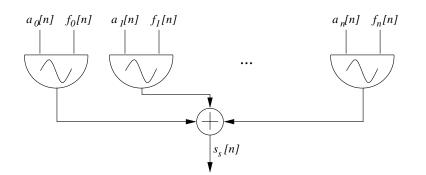
Figure 2.6: Sum of sinusoidal oscillators with time-varying amplitudes and frequencies.
