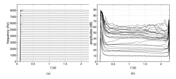
**Figure 2.8:** Fourier analysis of a saxophone tone: (a) frequency envelopes and (b) amplitude envelopes of the sinusoidal partials, as functions of time.
