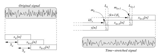
Figure 2.2: The generic SOLA algorithmic step.
