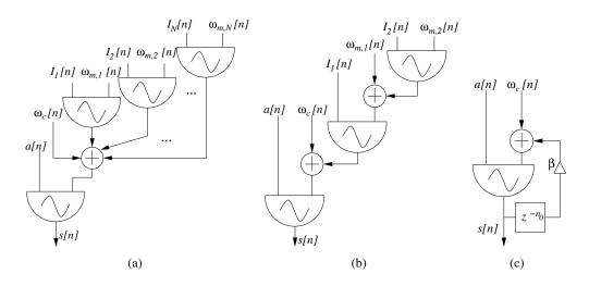
**Figure 2.36:** *Basic FM schemes; (a) compound modulation, (b) nested modulation, and (c) feedback modulation.*
