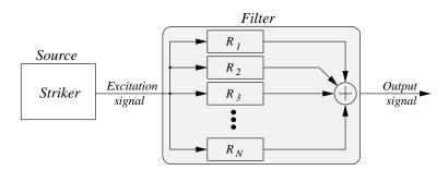
**Figure 2.19:** Parallel structure of digital resonators for the simulation of struck objects – the  $R_i$ 's have transfer functions of the form (2.28).
