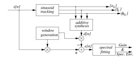
**Figure 2.10:** Block diagram of the stochastic analysis and modeling process, where s[n] is the analyzed sound signal and  $a_k$ ,  $f_k$ ,  $\phi_k$  are the estimated amplitude, frequency, and phase of the kth partial in the current analysis frame.
