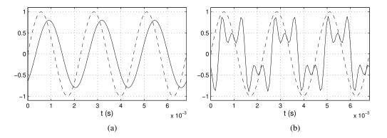
**Figure 2.29:** Example of output signals from a linear and from a non-linear system, in response to a sinusoidal input; (a) in a linear system the input and output differ in amplitude and phase only; (b) in a non-linear system they have different spectra.
