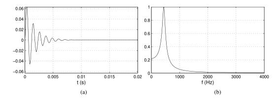
**Figure 2.18:** Example of a second-order resonator tuned on the center frequency  $\omega_c = 2\pi 440/F_s$  and with bandwidth  $B = 2\pi 100/F_s$ ; (a) impulse response; (b) magnitude response.
