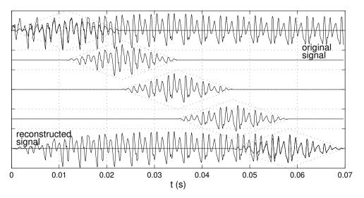
Figure 2.1: An example of OLA signal reconstruction, with triangular windowing.
