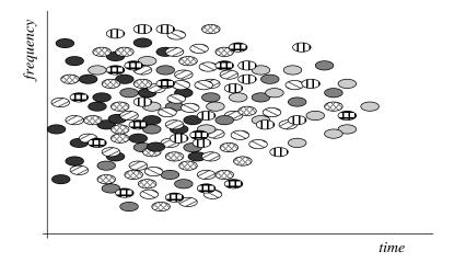
**Figure 2.4:** Representation of granular synthesis where grains derived from different sources are randomly mixed.
