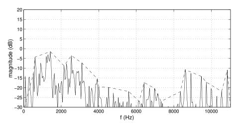
**Figure 2.11:** Example of residual magnitude spectrum (solid line) and its line-segment approximation (dashed line), in an analysis frame. The analyzed sound signal is the same saxophone tone used in figure 2.8.
