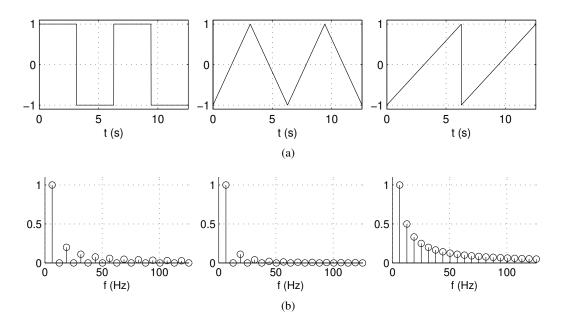
**Figure 2.16:** Spectrally rich waveforms: (a) time-domain square, triangular, sawtooth, and impulse train waveforms; (b) corresponding spectra (first 20 partials).
