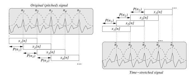
Figure 2.3: The generic PSOLA algorithmic step.
