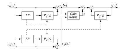
**Figure 2.27:** Block scheme of a LP-based implementation of cross-synthesis (also known as vocoder effect) between two input sounds  $s_1$  and  $s_2$ .
