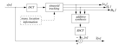
**Figure 2.14:** Block diagram of the transient analysis and modeling process, where s[n] is the analyzed sound signal and  $a_k$ ,  $f_k$ ,  $\phi_k$  are the estimated amplitude, frequency, and phase of the kth DCT-transformed transient in the current analysis frame.
