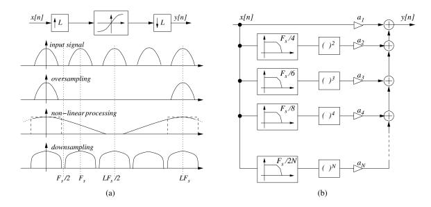
**Figure 2.31:** Two implementations of a memoryless non-linear system; (a) non-linear processing inserted between oversampling and downsampling; (b) non-linear processing on band-limited versions of the input.
