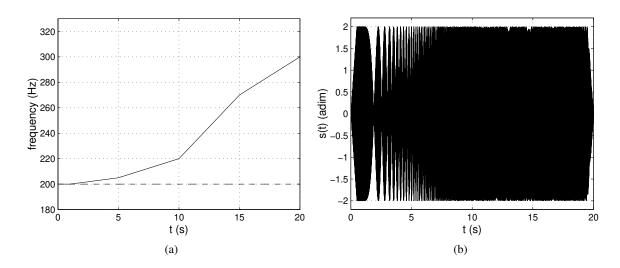
**Figure 2.7:** *Beating effect: (a) frequency envelopes (*f1 *dashed line,* f2 *solid line) and (b) envelope of the resulting signal.*
