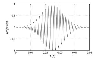
**Figure 2.5:** *Example of a synthetic grain waveform, with frequency*  $\omega_k = 2\pi \cdot 500$  *rad/s and standard deviation*  $\sigma = 0.2$ .
