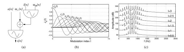
**Figure 2.35:** Simple modulation: (a) block scheme; (b) the first 10 Bessel functions; (c) spectra produced by simple modulation with  $\omega_c = 2\pi700$  Hz,  $f_m = 2\pi100$  Hz, and I varying from 0.5 to 3 (for the sake of clarity each spectrum is plotted with a different offset).
