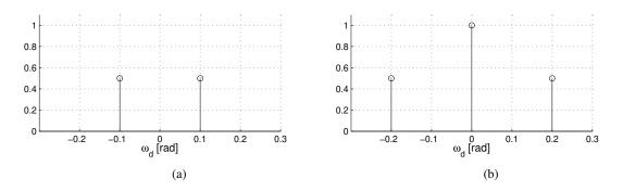
**Figure 2.30:** *Example of quadratic distortion; (a) spectrum of a sinusoid* x[n] *and (b) spectrum of the squared sinusoid*  $x^2[n]$ .
