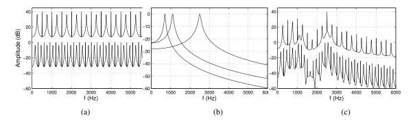
**Figure 2.22:** Formant synthesis of voice: (a) spectra of two pulse trains with fundamental frequencies at 150 Hz and 250 Hz; (b) first three formants of the vowel /a/; (c) spectra of the two output signals obtained by filtering the pulse trains through a parallel combination of the three formants.
