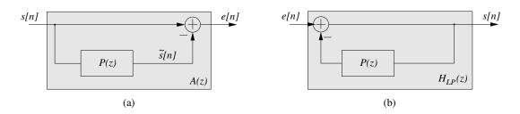
**Figure 2.23:** *LP* analysis: (a) the inverse filter A(z), and (b) the prediction error e[n] interpreted as the unknown input gx[n].
