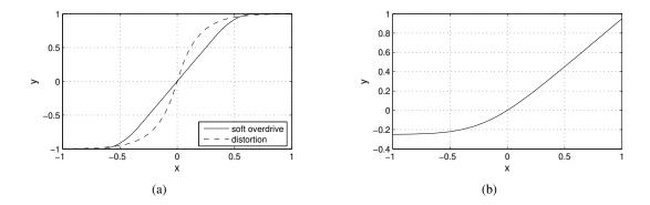
**Figure 2.32:** Simulation of overdrive and distortion; (a) soft overdrive and exponential distortion (with q = 6); (b) asymmetric clipping (with q = -0.2 and d = 8).
