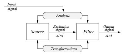
Figure 2.15: Source-filter model.
