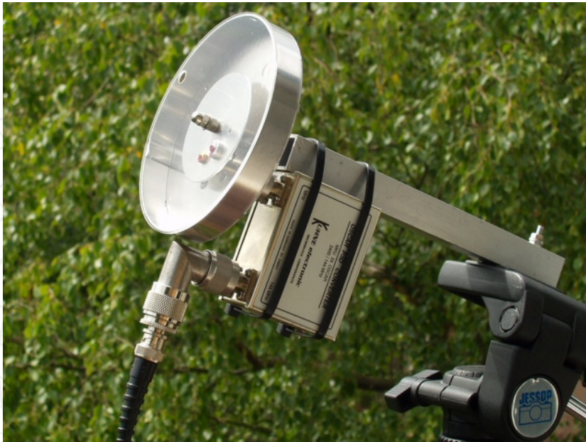
Small antenna RHCP patch G = 8.5 \text{ dBi} , \theta_{-3\text{dB}} = 90^\circ
