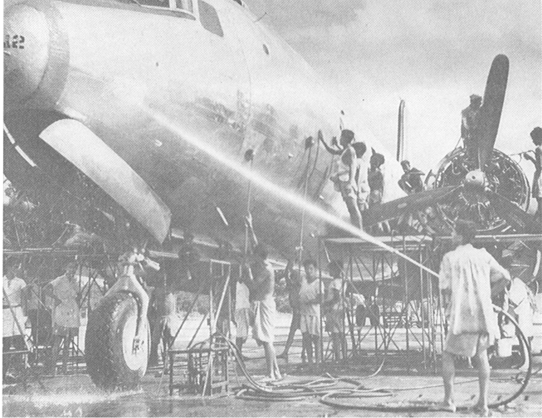
This veteran C-54 shows the effects of the much publicized—and severe —“Hump” weather. No amount of washing could remove the dimples caused by heavy hail on the skin of the aircraft. Serial numbers were often peeled off.
