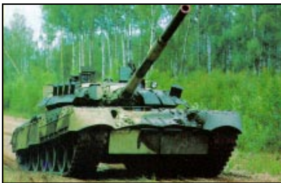
The T-80 designers unsuccessfully adopted a turbine engine, dropped later for unreliability and poor fuel economy. It also shared the T-72’s autoloader, a major vulnerability.
