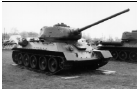
The T-34-85, with its 85mm cannon, went into production in 1944. The strength of the T-34 design allowed a weight increase of 23 percent without reduced effectiveness.
