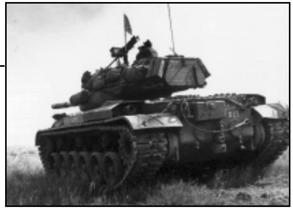
A gasoline engine limited the range of the M47, above. Most were exported. Instead, the U.S. adopted the diesel-powered M48, below.
