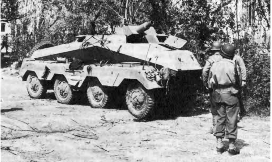
8 RAD PANZERSPAHWAGEN, mounting the 7.5-cm. short-barreled gun.
