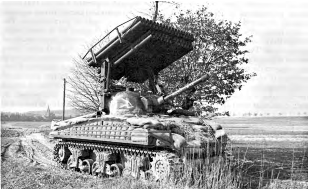
MULTIPLE ROCKET LAUNCHER T34 mounted on a Sherman tank.
