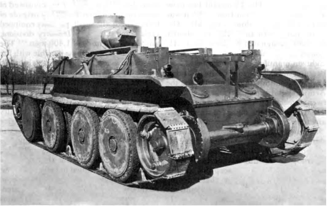
MEDIUM TANK T3, one of the Christie tanks.
