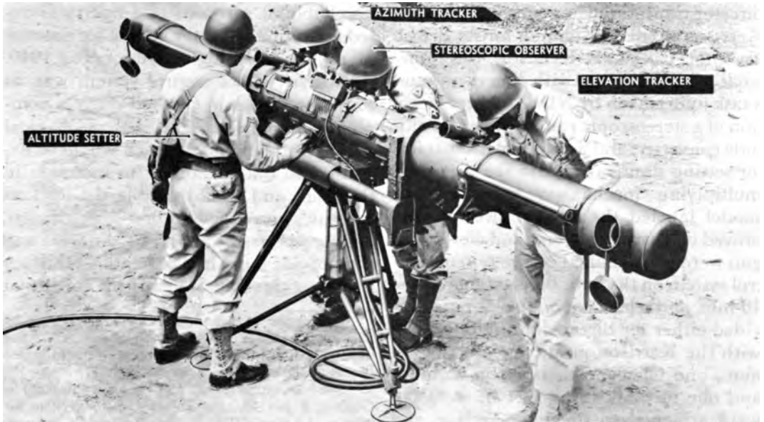
FIRE CONTROL INSTRUMENTS. Director T30 (above) and height finder M1 (below).
