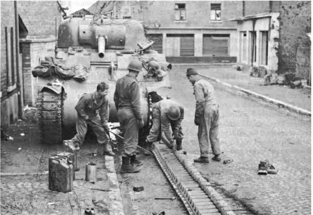
TRACK EXTENSIONS being installed by the crew of a Sherman tank during a lull in combat operations at Baesweiler, Germany.
