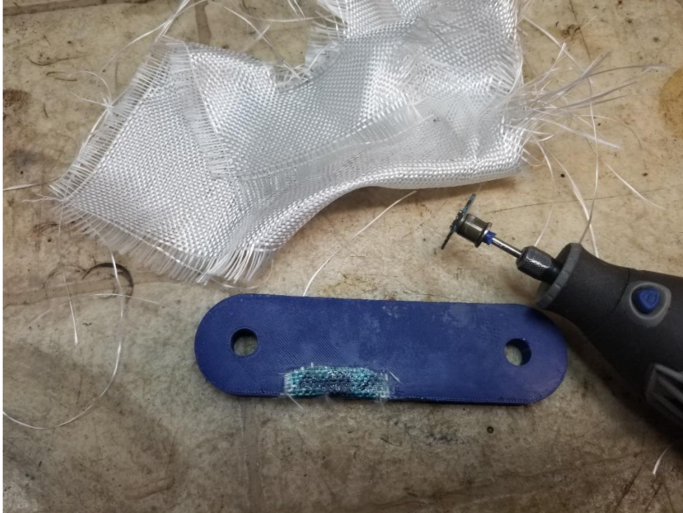
Figure 14: Excess fiberglass cut away
