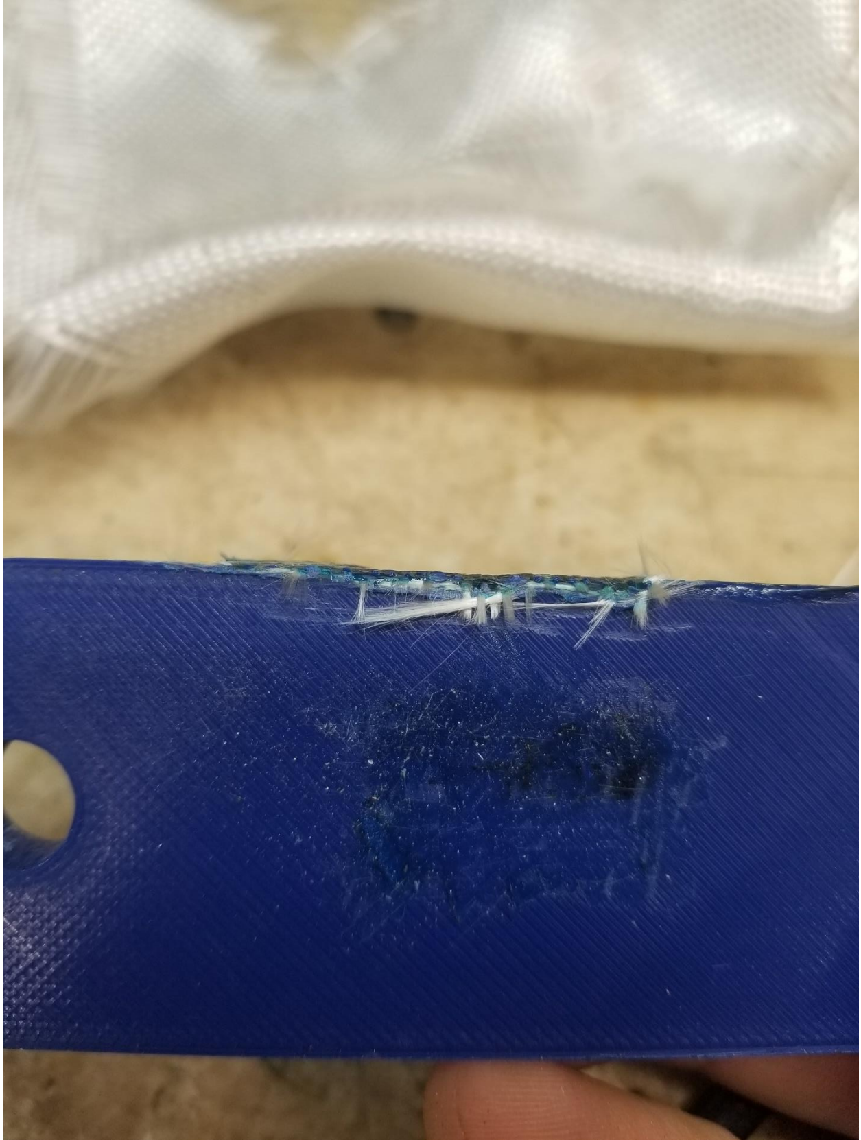
Figure 15: A look at the relative straightness of the part maintained after heat-welding.
