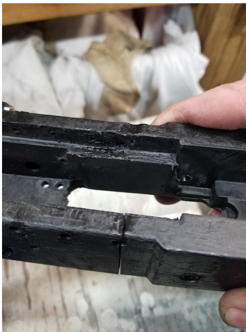
Figure 2: Plastikov receiver cracked along an area that was not re-melted
