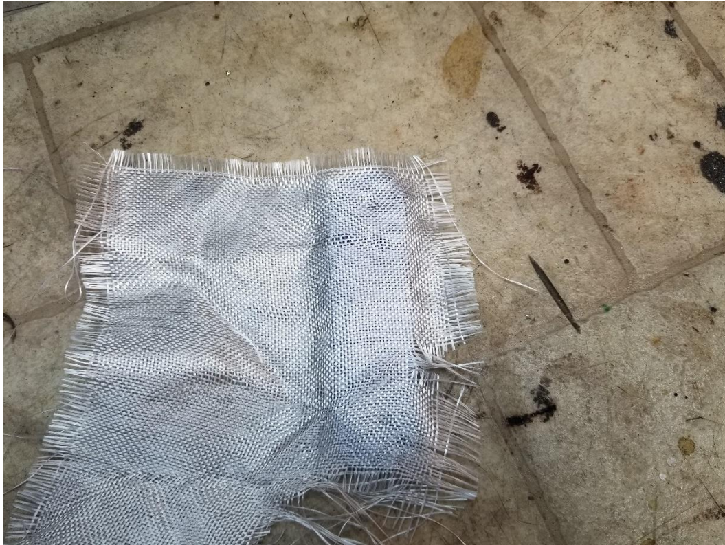
Figure 10: Fiberglass sheet drawn tightly over the part. As you move to melt plastic into it, hold it tight - clamps may help you.
