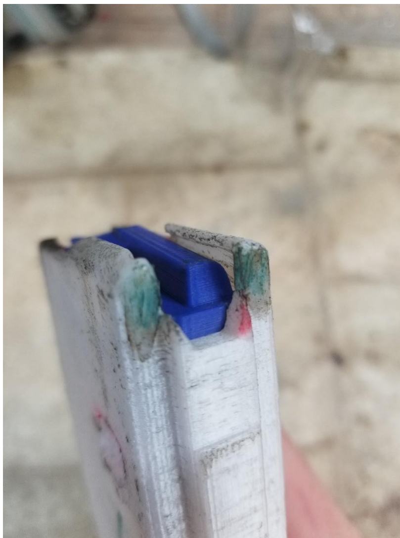
Figure 1: AR15 magazine with re-melted feed lips shown in green
