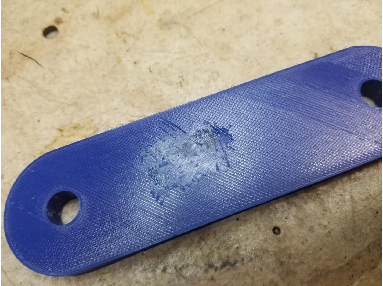
Figure 7: Another example spot re-melted - note the disappearance of layer line pattern.
