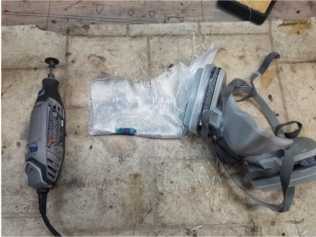
Figure 12: Note the appearance of the heat-welded spot. The blue plastic has soaked into the fiberglass in the area treated.
