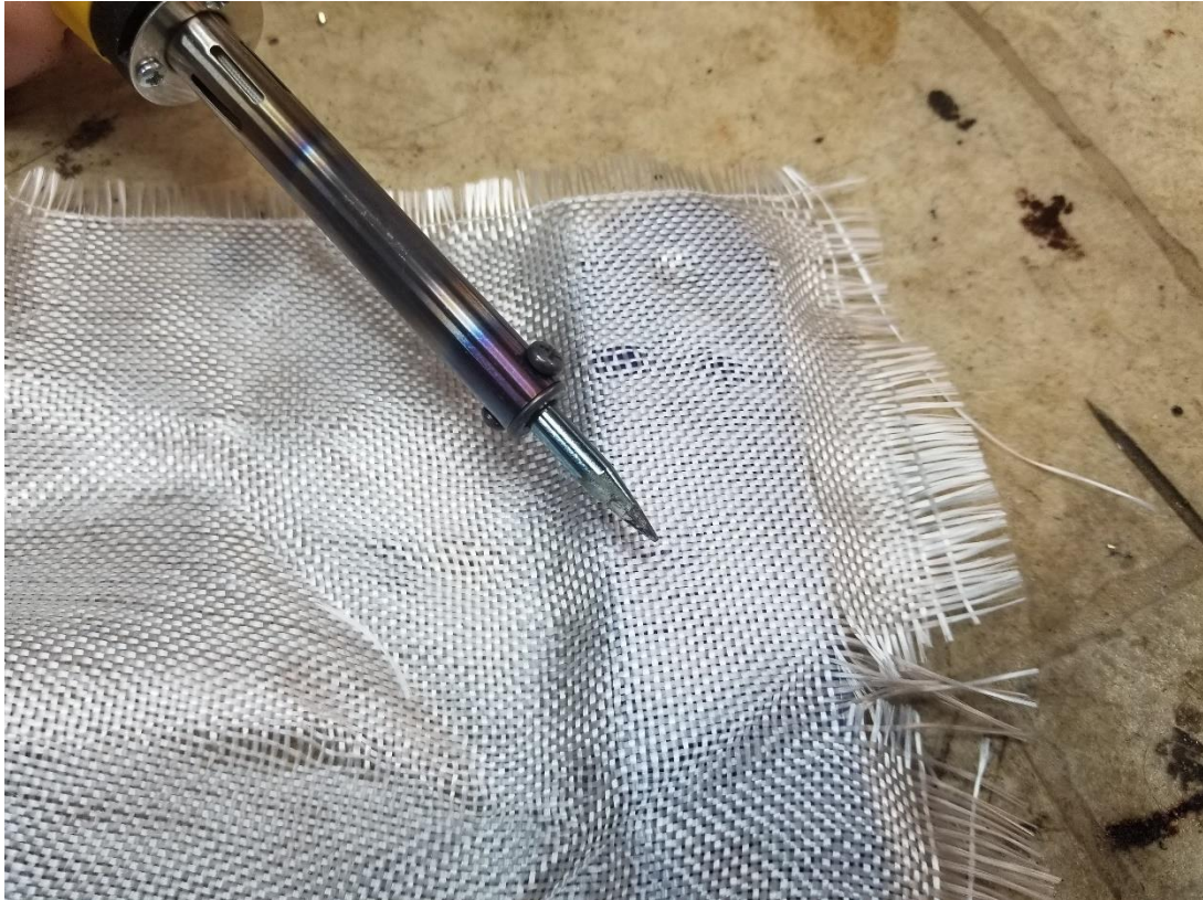
Figure 11: As with re-melting, gently press the soldering iron onto the part.
