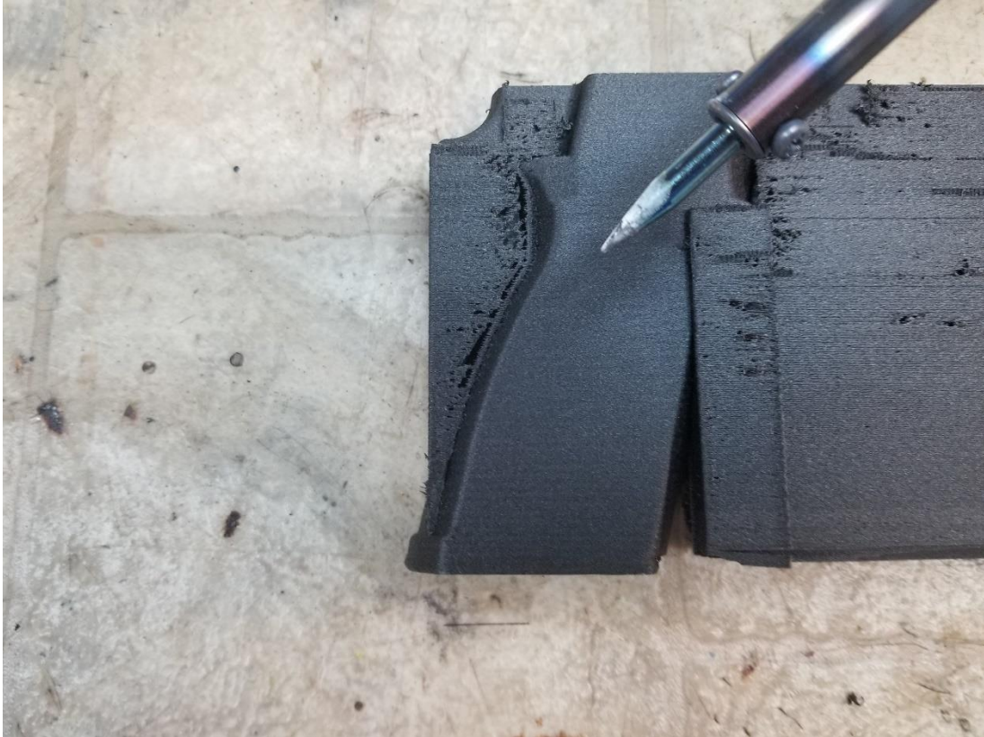
Figure 4: Printed part ready to be re-melted. Usually you would remove supports before this process.
