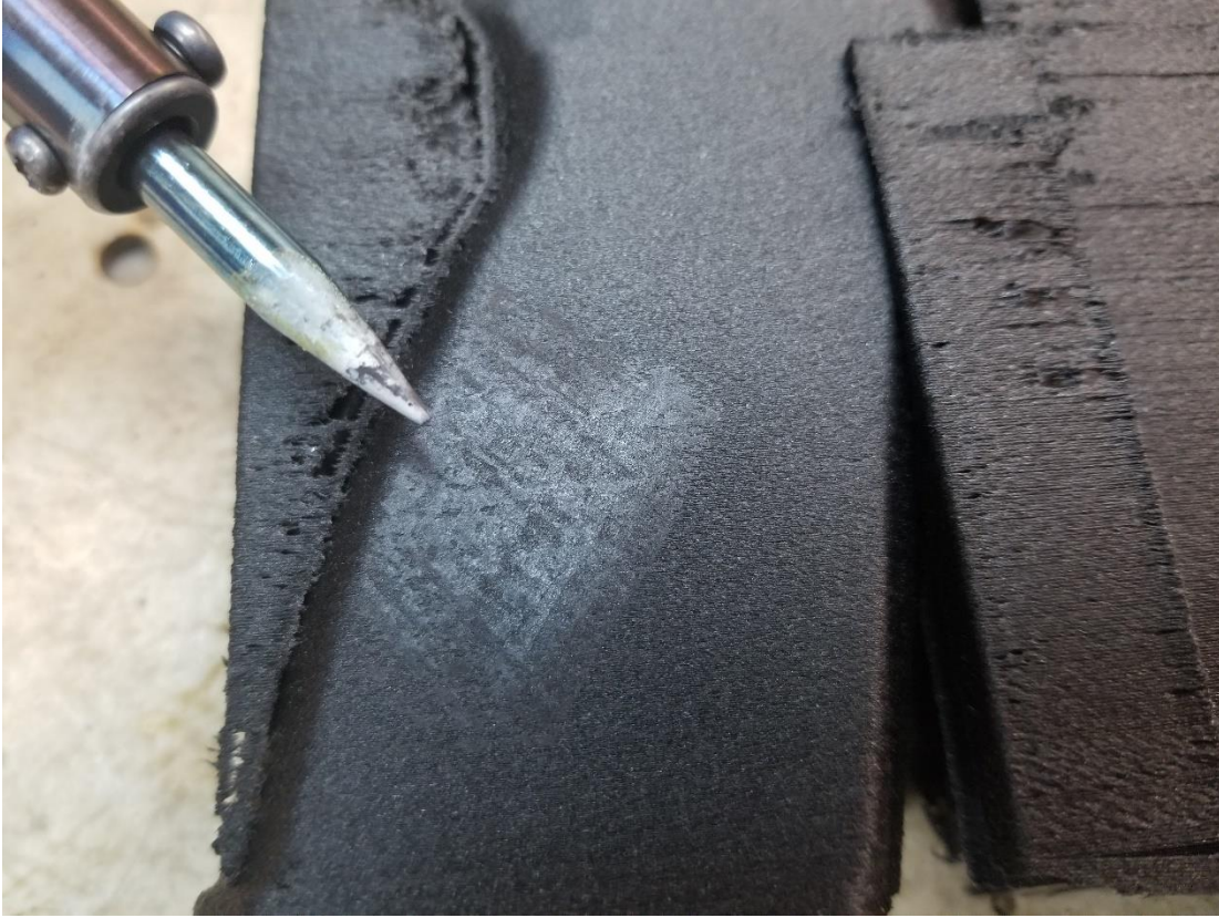
Figure 5: Example of a spot re-melted. Note the change in surface appearance and disappearing of layer line pattern.
