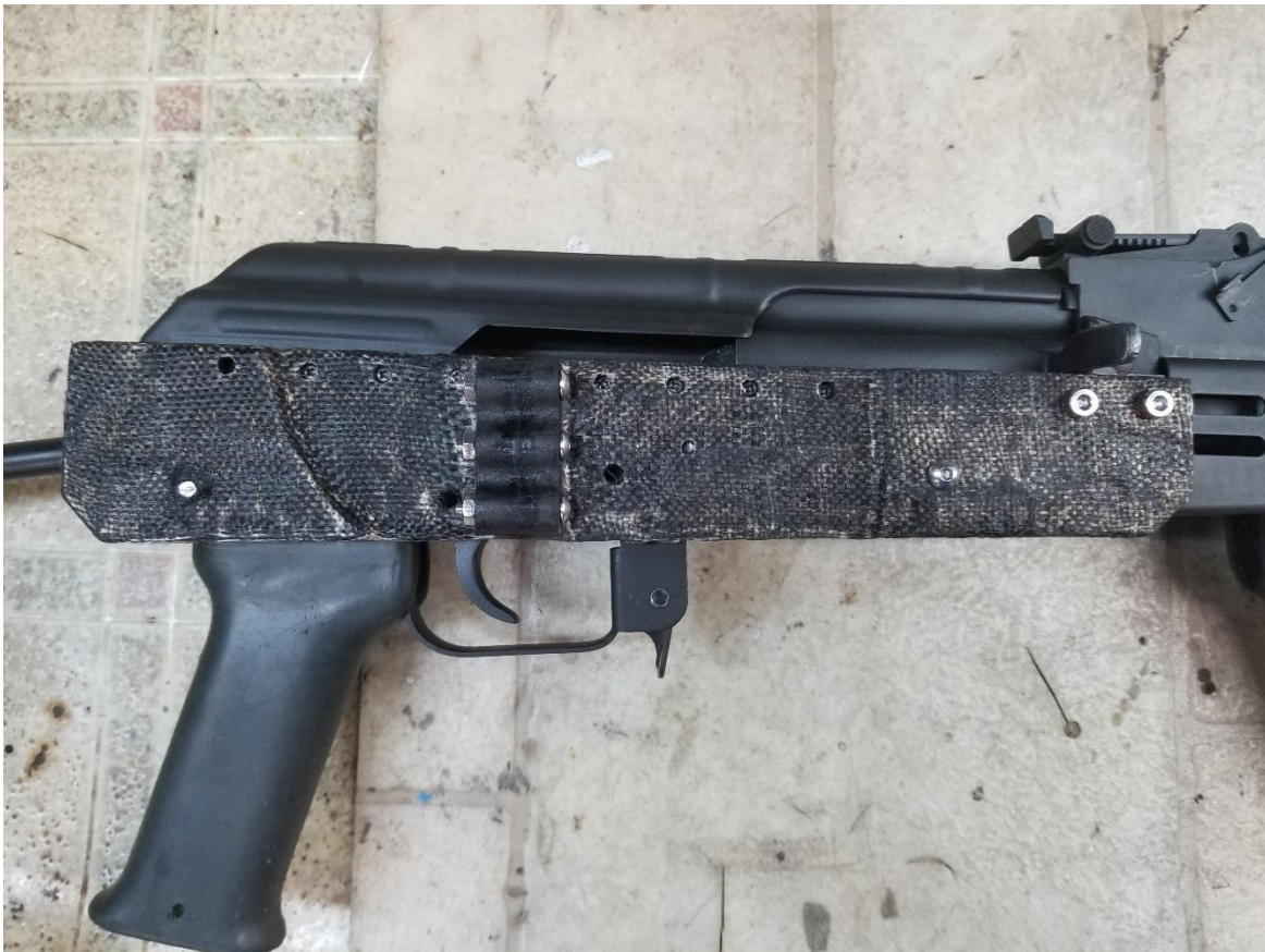
Figure 3: Plastikov Receiver with full fiberglass helt-weld wrap
